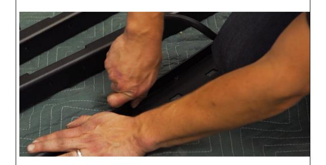
5. Fit Pinch weld to short edge of roof rails. Trim excess off with side cutters.
