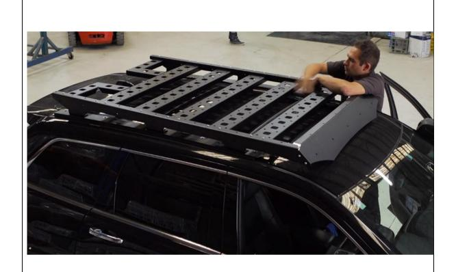
16. Loosely fit M8 bolts spring washers and washers through rack into nutserts fitted to steel rail.
