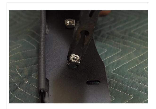
6. Fit nutserts as shown in both rails (6 per rail). You can use needle nose pliers or screwdriver to push one end of cage in from side.
