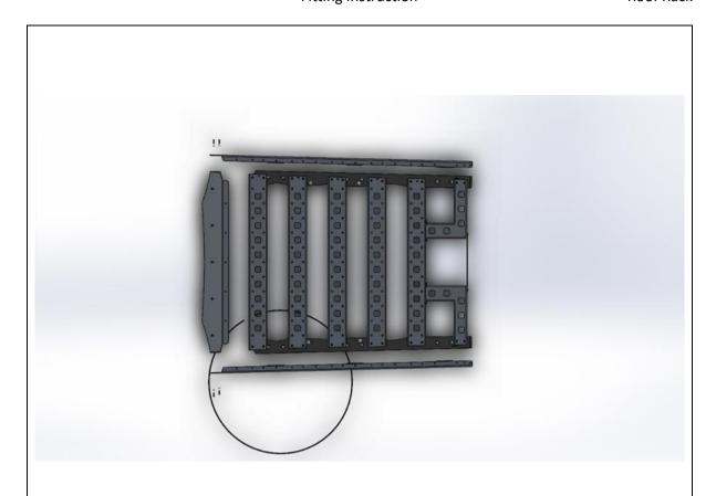
Lay all parts out as shown ready to be bolted together. Panels are labeled with numbers 1-5, with 1 being towards the front. As can be seen, the entire rack is dove tailed to suit Jeeps roof. Front is wider than back. **TOOLS REQUIRED**
